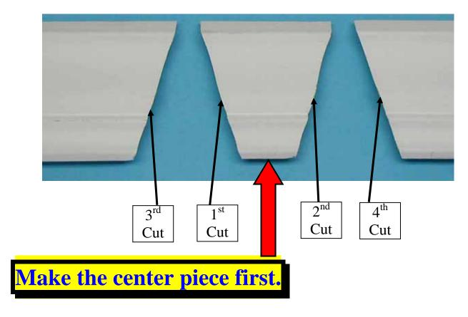
**Cut** #1 is an outside corner RH, horizontal cut and is cut just like the example on page 30,  $2^{nd}$  photo. From Table 1, page 55, your true corner angle is  $225^{\circ}$  (see page 53, last drawing) .... and your horizontal turn crown slope angle is  $52^{\circ}$ ...... from the crown molding table on page 36, your saw settings are: **Miter = 14.3°**, **BT = 17.6°**
